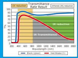
It reduces the transmittance of radiation from outside thus you can adjust the temperature of the air conditioner 2-3 °C higher. In contrast, it reduces the transmittance of radiation from the inside during winter thus the temperature of the heater can be set lower.
